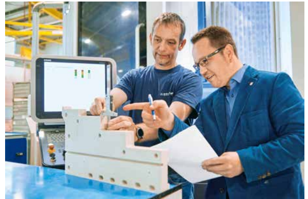
— CNC milling technician Heinz Tieben (on the left) and Frank Dickmann, Head of Quality Management in Haren, use a vernier caliper to determine the contour accuracy.
