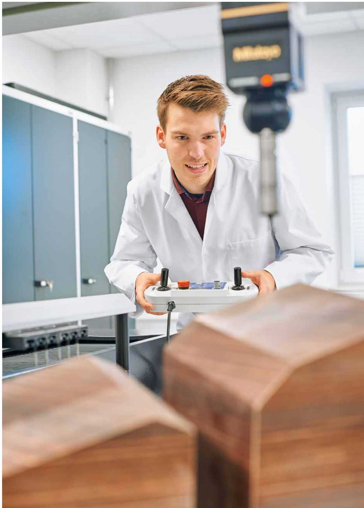
— Andre Hackmann is the quality assurance officer for the machining of composites in Haren. The 3D coordinate measuring machine that he works with uses a tactile measurement sensor, making it possible to measure parts accurately down to hundredths of a millimeter.
