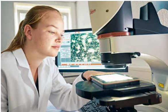
— Helena Meyer, apprentice process mechanic for plastic and rubber, uses a digital microscope to check the quality of a material chip from a pressed sheet.
