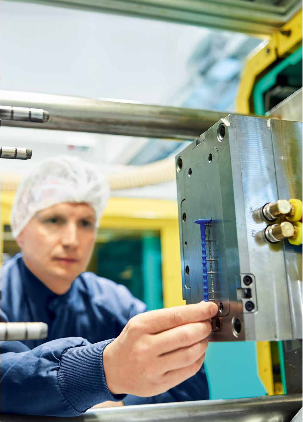
— Dimitri Dering, an applications engineer in the production department in Brensbach, Germany, at an injection-molding machine used to manufacture the oral syringe for the Sympfity system. Röchling has developed a tool prototype that is being continuously optimized.
